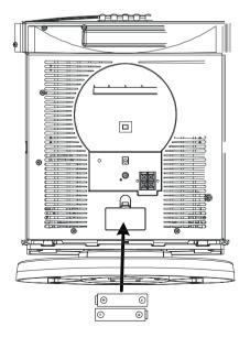
Remember to replace the battery compartment lid 3 "AA" size batteries
